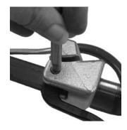
3. Replace pin: Align gripper hole with slide block hole, insert pin in hole and hammer pin in place.
