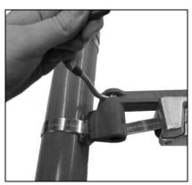
6. Pull cutting handle to cut the band. When applying Giant Band clamps, prior to cutting off clamp, release band gripper and push tool nose away from buckle approx. '4".
