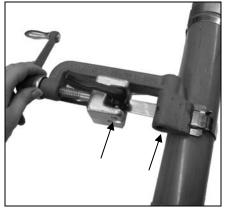
3. Place band in open of tool nose and gripper block. Move into slot as far as possible, to avoid buckle sliding into tool nose. Apply tension by turning handle of tool
