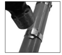
8. Hammer down buckle ears to complete BAND-IT clamp.
